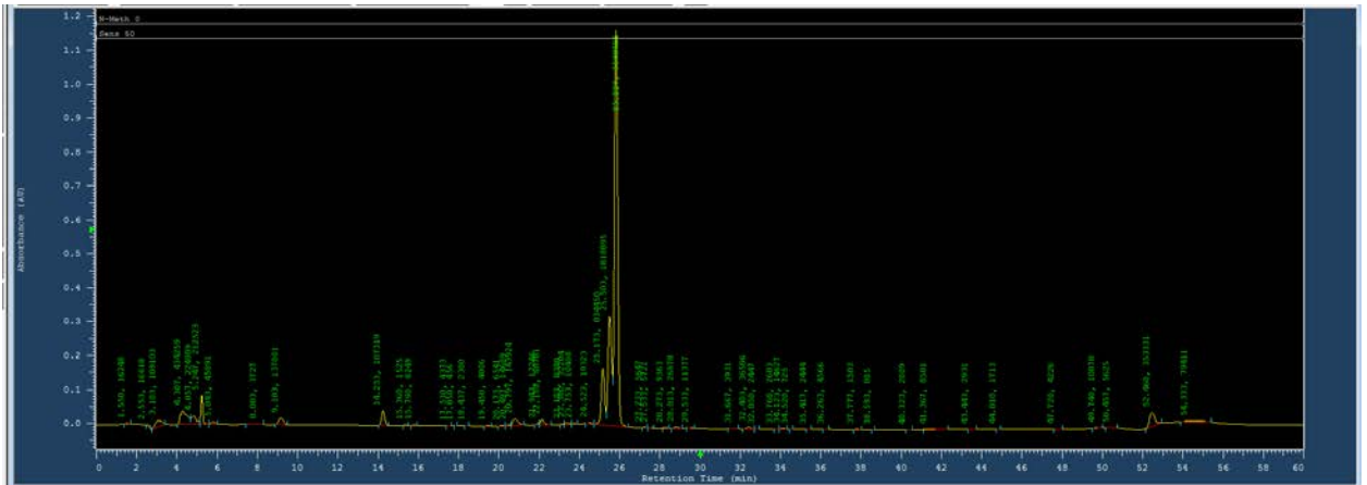
Figure 9. HPLC chromatogram from a pure Curcumin sample diluted in methanol (Ideal wavelength: 200 nm)
